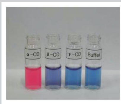
Photograph of the polydiacetylene liposomes after 1 h in the presence of 10 mM of the three different cyclodextrins in a HEPES buffer solution.
